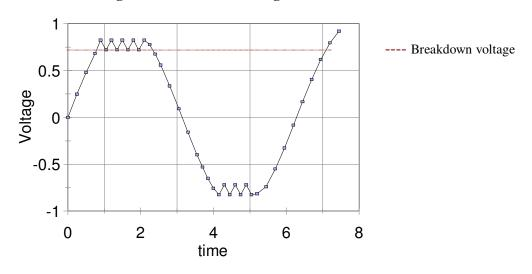
Voltage curve in a DBD discharge cell
